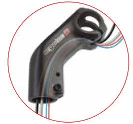
interne Kabelführung / internal cablerouting Faceplates S./P. 118/119
